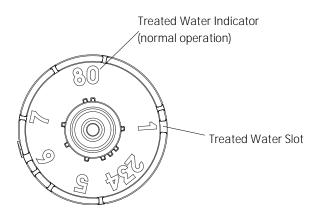
The corresponding slot for the number is positioned at the optical sensor which is approximately 90 degrees out of phase.
