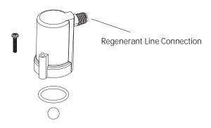
Figure 11 Regenerant Connection for Performa Valve
