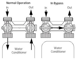
Figure 7 Typical Globe Valve Bypass System
