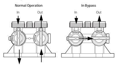
Figure 6 Series 1265 bypass for use with Performa valve bodies
