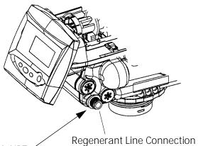
**NOTE:** Be sure to use a 3/8 inch NPT plumbing connection when attaching regenerant line to the Performa valve.
